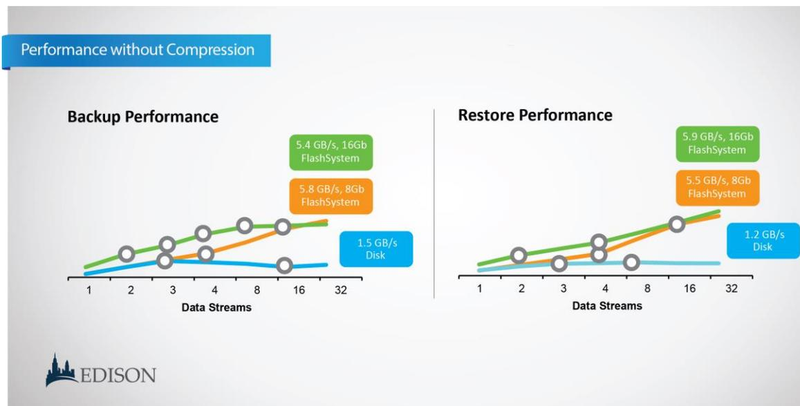
Figure 6: SD 5.0 performance with FlashSystem vs disk, without compression
