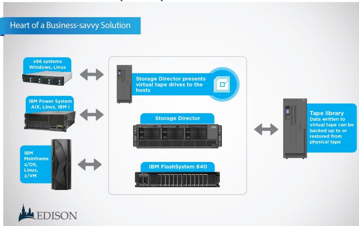
Figure 4: Tape at the speed of flash solution architecture
